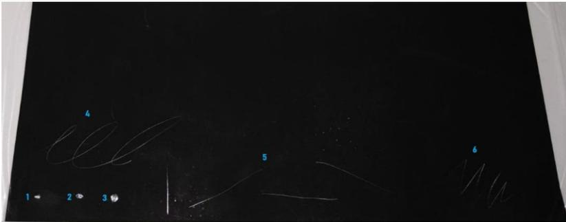
The layers of are about 10 microns thick and are applied on top of each other on a carrier foil of about 30 centimetres wide in a continuous roll-to-roll process, moving the foil at speeds up to 1 m/s. To ensure proper application, possible imperfections like variations in thickness and the absence of holes in the membrane and catalyst layers must be correctly detected and measured.
