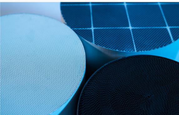
They wanted to detect any abnormalities in the catalyst's coating, such as lumps or coating thickness that could result in a low-quality product that would be rejected by their customers, or just managing the process and keeping an eye on the dosing consumption and process efficiency, and avoiding scrap. With DPFs, the optical leaks were a major concern, as any leak could mean that not only the light but also particles could pass the filter and would reach the atmosphere.
